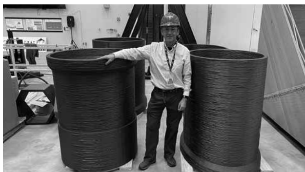
Above: Printing the TIDC-designed culvert diffuser in the ASCC lab. Below: Dr. Roberto Lopez-Anido, TIDC lead researcher, with 3D printed diffuser sections. The diffusers are being piloted at two locations: Thorndike, Maine; and Exeter, New Hampshire.
