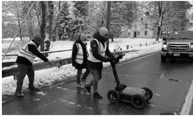
Above: Students from University of Massachusetts-Lowell use electromagnetic detection to identify concrete cracking for a project using the technology to assess highway bridges. Below: A student from University of Vermont performs a stream network assessment to identify sensitive structural, hydraulic, and landscape parameters for flood mitigation planning.
